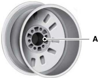
A Hub pilot bore.
