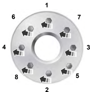
8-lug nut torque sequence
