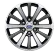
XLT 18" Machined-Face Aluminum with Magnetic-Painted Pockets Standard
