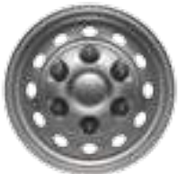
16" Silver Steel with Exposed Lug Nuts Standard: Heavy-Duty Front Axle SRW
