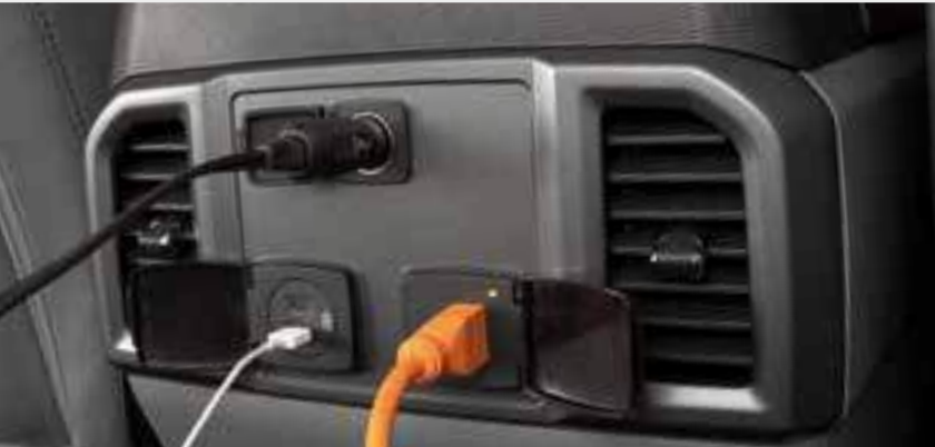
100V/400W AC POWER OUTLET ON CENTER CONSOLE REAR (SuperCab/Crew Cab) Standard on LARIAT; Available on XLT
