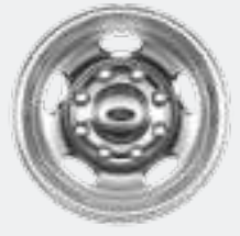
17" Polished Forged-Aluminum with Bright Center Cap 3 Standard: F-350
