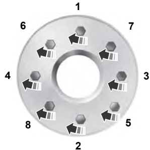
8-lug nut torque sequence
