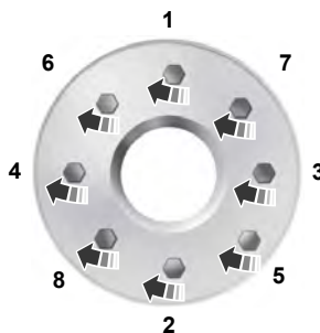
8-lug nut torque sequence
