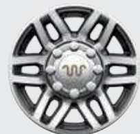
18" Bright-Machined Cast-Aluminum with KING RANCH Center Cap Standard: F-250/F-350 SRW KING RANCH
