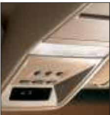
The new overhead console includes individual map lights, a compass, valet clip and sunglass storage.
