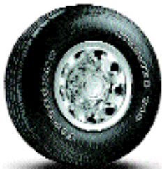
16" polished aluminum wheel. LT265/75Rx16 OWL All-Terrain tire. Optional on XLT.
