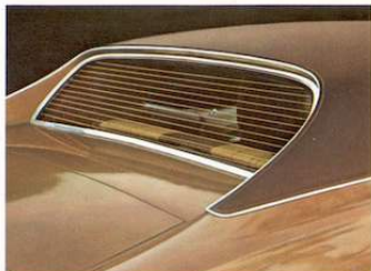
ELECTRIC REAR WINDOW DEFROSTER Thin conductive strips in the backlite warm up to improve rear visibility. Includes tinted glass. Available on all models except Convertible.
