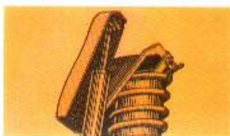
FRONT OVERLOAD AIR SPRINGS . . . Overload air springs may be installed in the front coil springs of your Bronco for increased capacity and for snowplow service.
