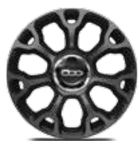
17-INCH 7-SLOTTED- SPOKE MATTE BLACK PAINTED MACHINED ALUMINUM Available on Trekking with Urbana Appearance Package
