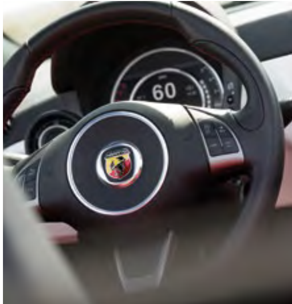
Three-spoke leather-wrapped steering wheel with a race-style flattened bottom intended for track and street.
