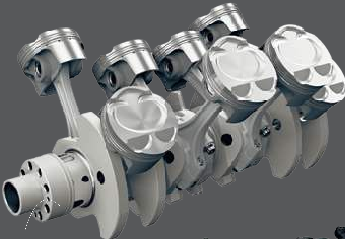
Pistoni forgiati e albero piatto Forged pistons and flat crankshaft
