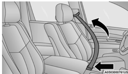
Positioning The Lap Belt
