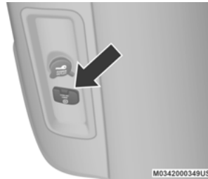
Power Inverter Outlet
