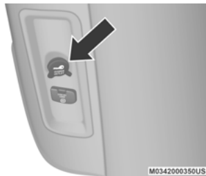
Rear Panel Power Outlet
