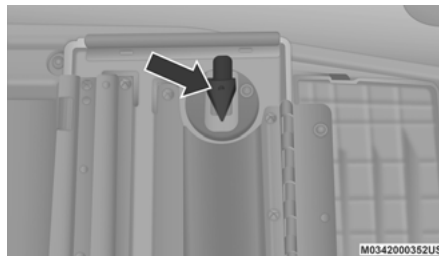
Storage Bin Cover Emergency Release Lever
