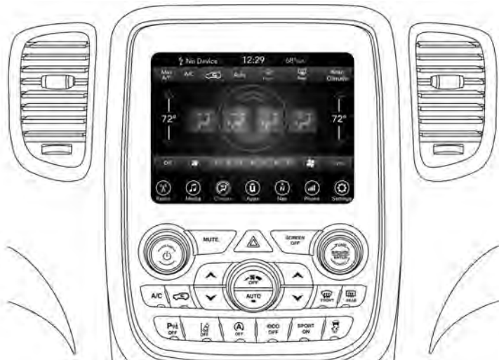
Uconnect 4C/4C NAV With 8.4-inch Display Temperature Controls
