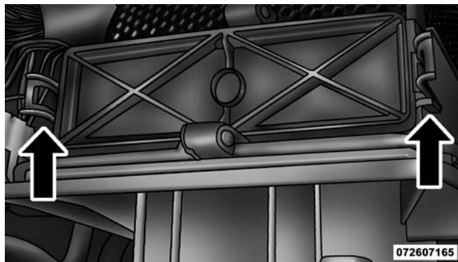
A/C Air Filter Replacement
