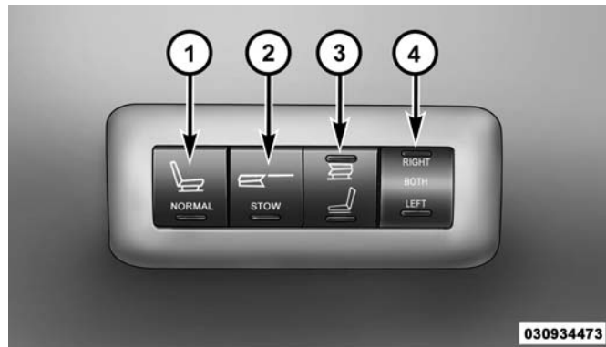
Rear Panel Power Switch Bank
