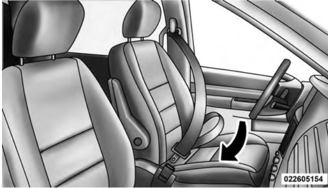
Inserting Latch Plate Into Buckle
