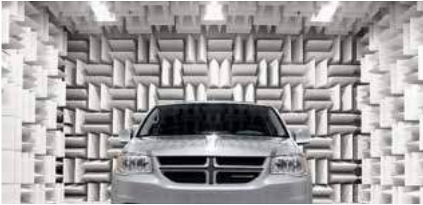
ANECHOIC CHAMBER — NOISE, VIBRATION AND HARSHNESS (NVH) TESTING
