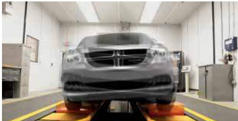
FOUR-POST SHAKER — SUSPENSION TESTING
