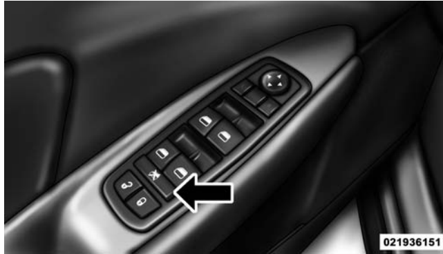
Window Lockout Switch
