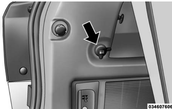
Rear Cargo Area Power Outlet
