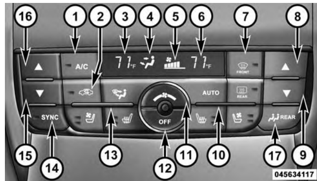
Automatic Temperature Control (ATC) Panel
