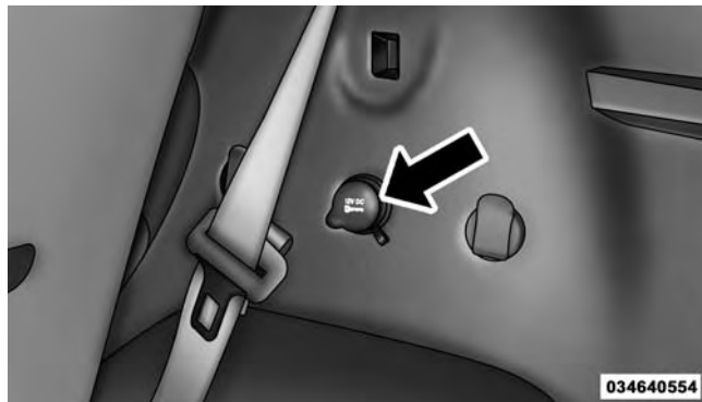
Rear Cargo Power Outlet
