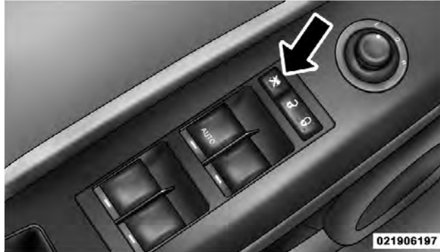
Window Lockout Switch
