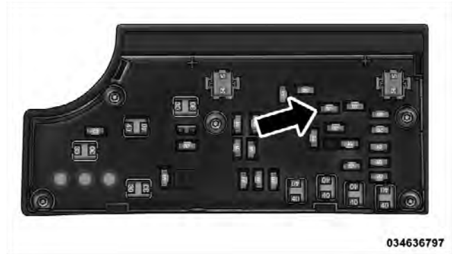
Power Outlet Fuse Location
