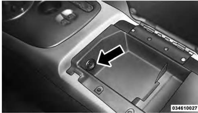
Center Console Power Outlet
