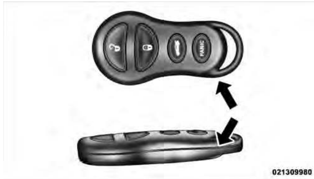
Separating RKE transmitter Halves
