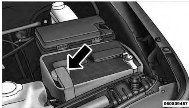
Positive Battery Post
