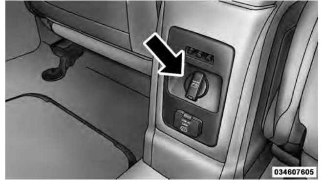
Rear Power Outlet
