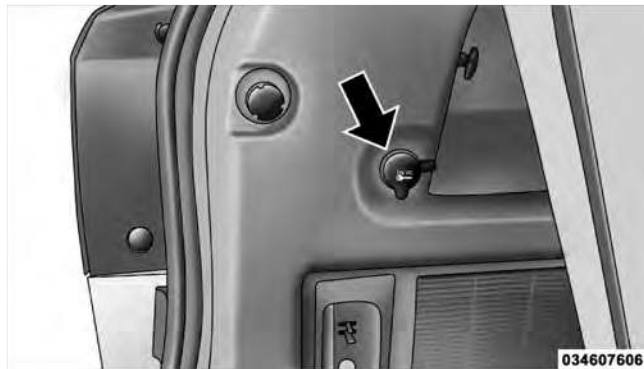
Rear Power Outlet
