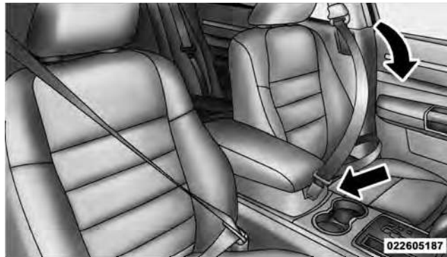
Removing Slack from Belt
