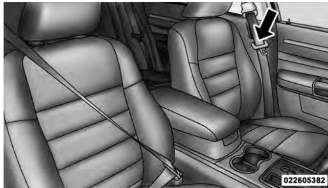
Pulling Out the Lap/Shoulder Belt Latch Plate
