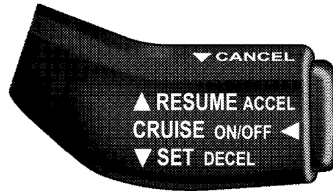
Electronic Speed Control Lever
