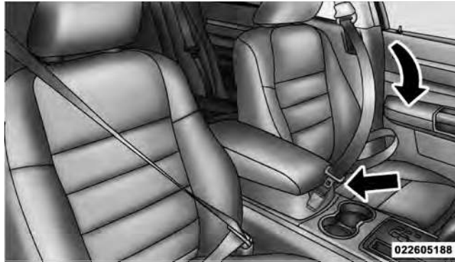
Inserting Latch Plate into Buckle
