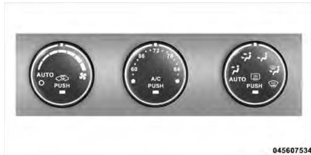
Automatic Temperature Control
