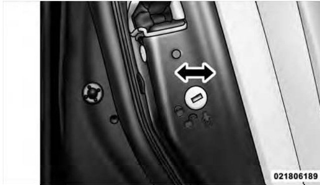
Child-Protection Door Lock Function
