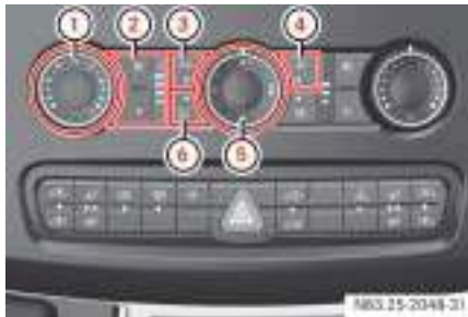
Control panel for the air-conditioning system
