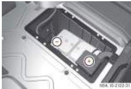
Starter battery in the driver's footwell
