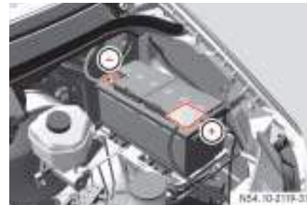
Auxiliary battery in the engine compartment
