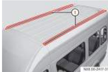
① Securing rails
