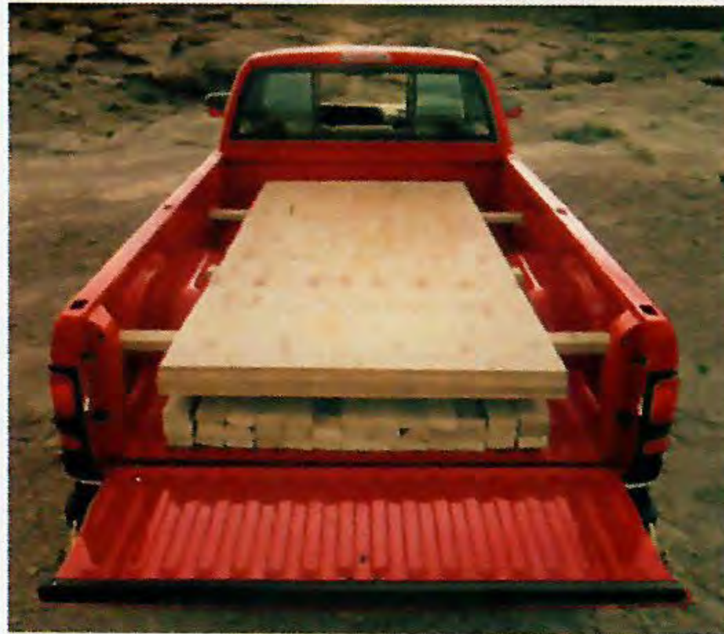
The RAM cargo bed is a versatile system of work features engineered for a variety of cargo hauling needs. Box side indentations hold 2x8 supports, creating a second level for two-tier loading. Pockets in the box sides allow insertion of vertical stakes for tall loads. ♦
