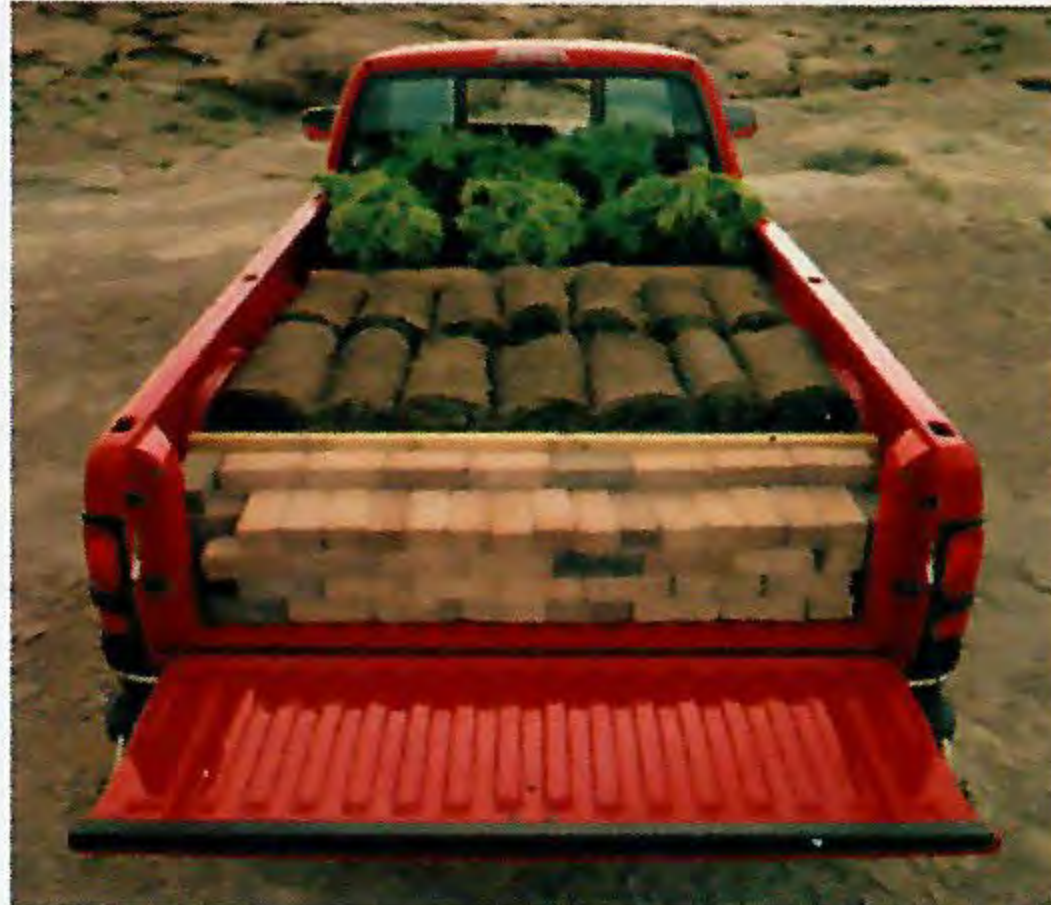
♦ Dodge-exclusive cargo bed provisions support 2x8 bulkheads that divide the bed into three loading compartments to prevent loads from shifting, and for separating and organizing cargo.
