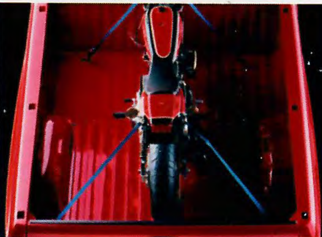
♦ Dodge-exclusive cargo tie-downs are widely spaced and anchored to the structural front-box support rail for extra strength. Front tie-downs are recessed into the box floor and concealed by snap-in plastic covers. Rear tie-downs are high-strength “U” brackets bolted to the base of each rear box corner.
