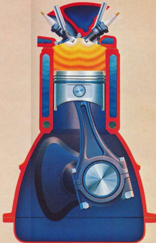
More power from less gas than the engine it replaced: the inner workings of the NAPS-Z engine.
