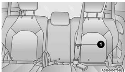
Routing The Rear Seat Belt Latch Plate
