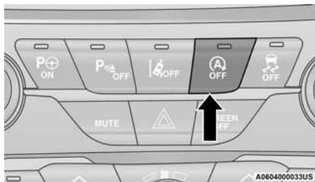
Stop/Start OFF Switch
