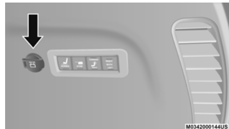
Rear Power Outlet
