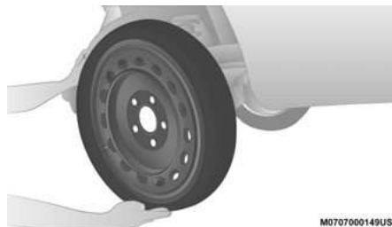
Mounting Inflatable Spare Tire
