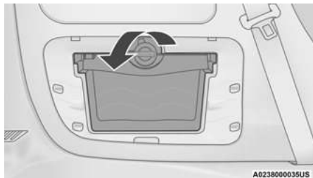
Debris Bin Release Knob
