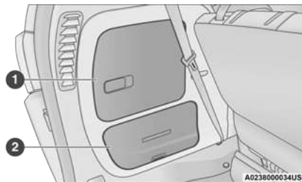
Vacuum System Access Panels
