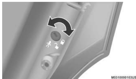
Child-Protection Door Lock Function
