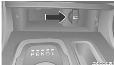
Front Power Outlet
