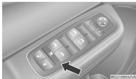
Window Lockout Switch
