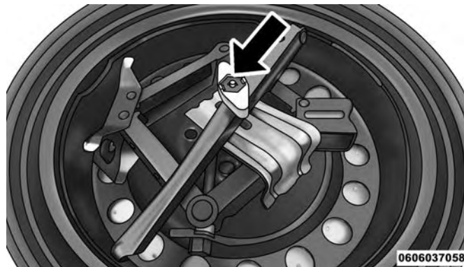
Jack And Spare Tire Fastener
