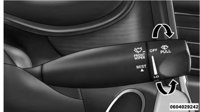
Windshield Wiper Operation
