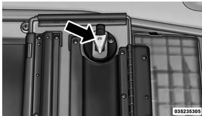
Storage Bin Cover Emergency Release Lever
