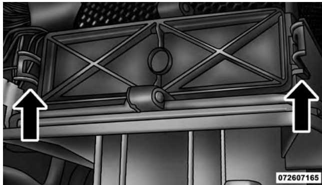
A/C Air Filter Replacement
