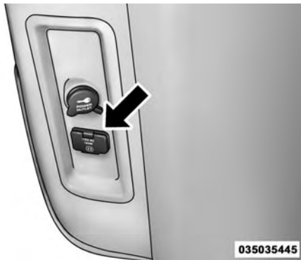
Power Inverter Outlet
