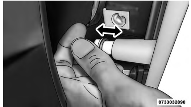
Front Side Marker Lamp Bulb Removal
