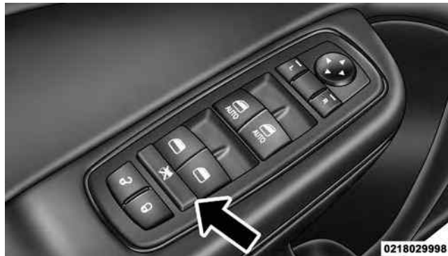
Window Lockout Switch
