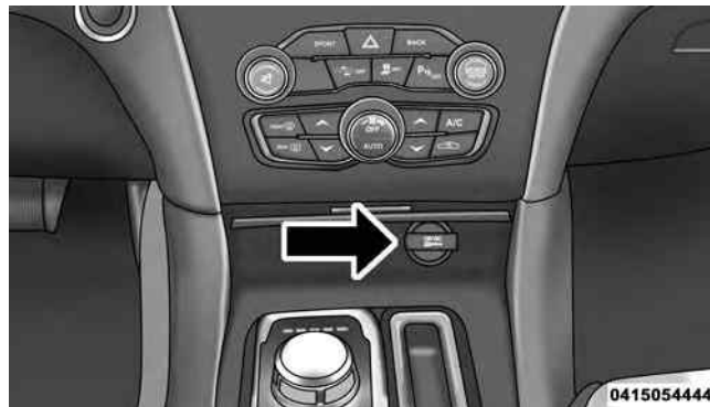
Front Power Outlet
