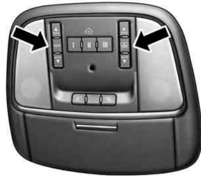
CommandView® Sunroof And Power Shade Switches
