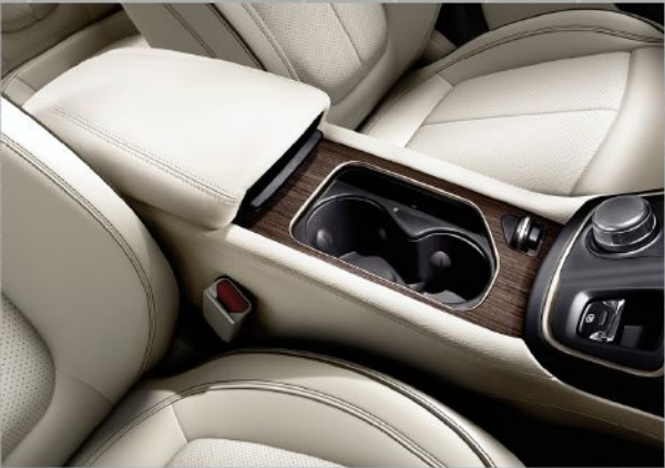
1 - 2 - 3: FULLY OPEN, HALF-OPEN AND FULLY CLOSED. The cup-holder tray can be slid to the half-open position if a single beverage container is in the forward cup-holder position. The sliding cup-holder tray makes way for additional storage beneath. The two-container cup holder is size-adjustable via rubberized gripping elements to ensure secure stowage of everything from a 12-ounce can to 1.5-liter bottle.
