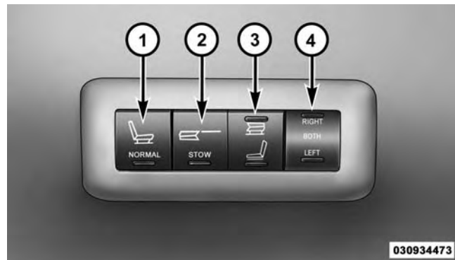
Rear Panel Power Switch Bank
