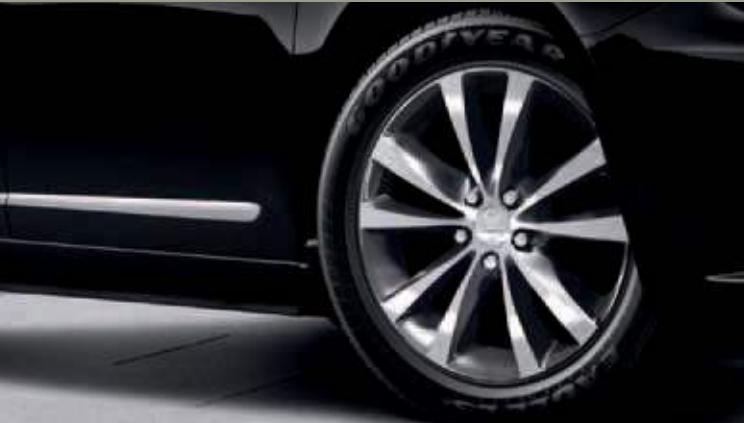
18-INCH POLISHED ALUMINUM WHEEL WITH BLACK PAINTED POCKETS Optional on Limited and Touring (with S Appearance Package).
