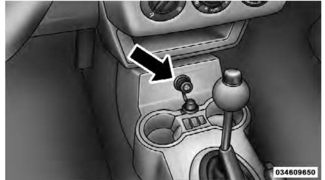
Front Power Outlet
