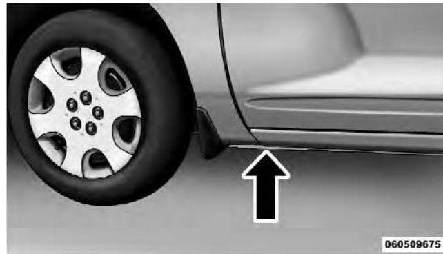
Front Jacking Location
