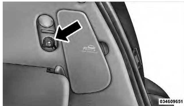
Rear Power Outlet
