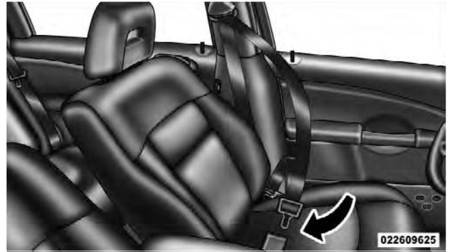
Inserting Latch Plate Into Buckle
