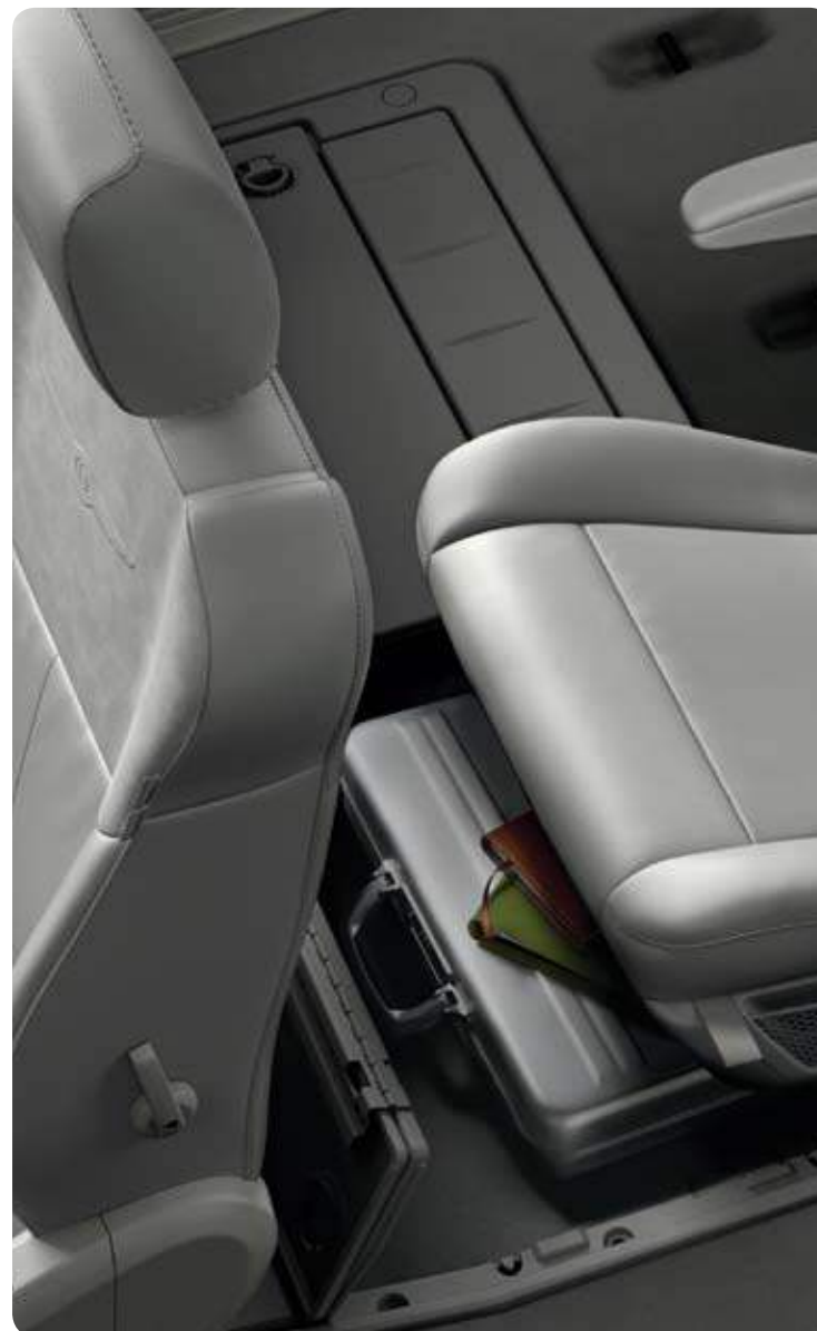
Second-row in-floor storage bins closed and open.
