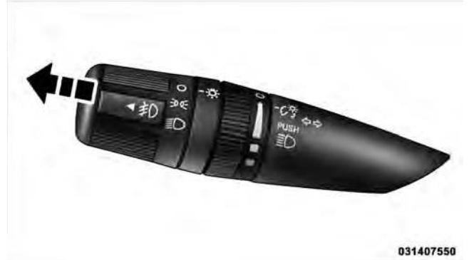
Front Fog Light Control
