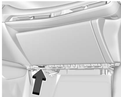
Interior Power Outlet
