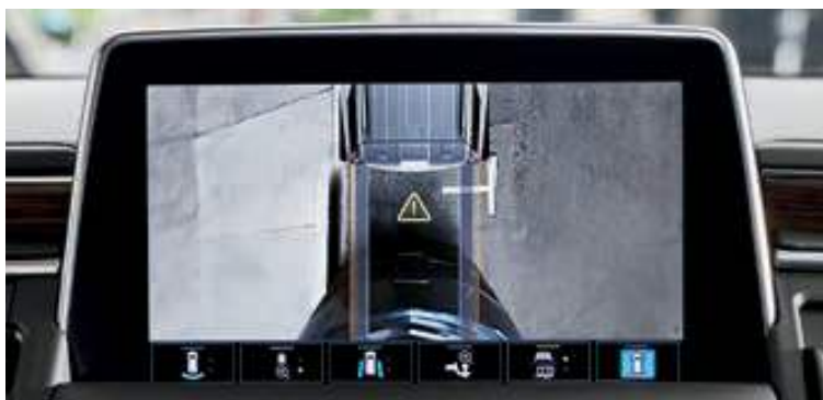
Rear Top-Down View Shows the clearance between the rear of the vehicle and nearby objects.
