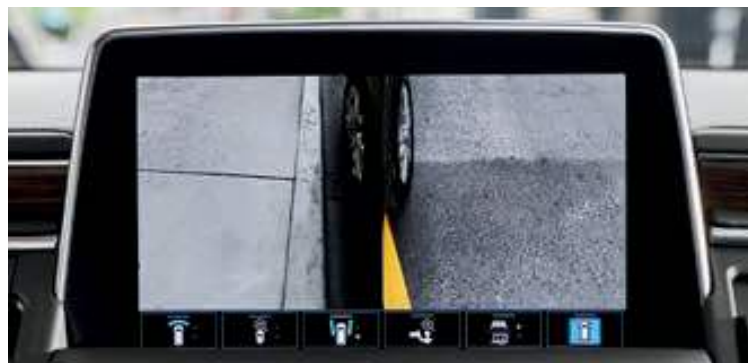
Rear Side View Provides a line of sight down each side of the vehicle.
