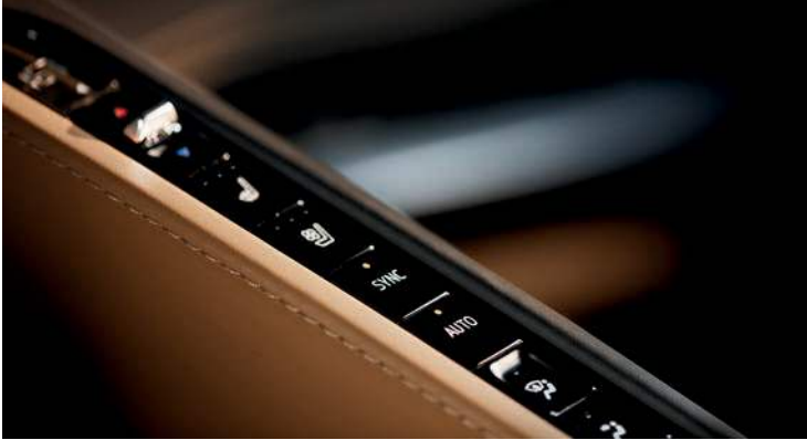
CLIMATE AND SEAT CONTROLS ATOP COCKPIT BUTTRESS
